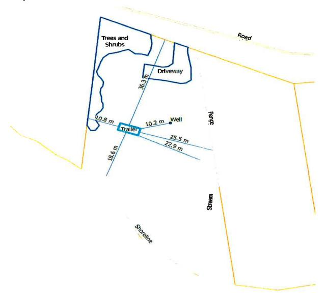
Sample only: your property may not have all of these features, but this site plan is intended to demonstrate the distances and setbacks to be shown. Please include any other structures or features and the distance from the trailer. A hand drawn site plan will be accepted.
