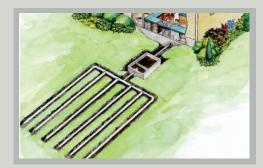
A licensed sewage hauler or onsite sewage system professional should remove the septic tank cover and inspect the system every three to five years and pump out the solids and scum when required.
